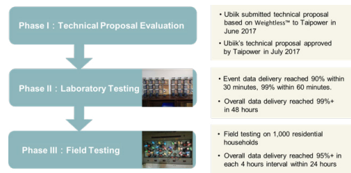
Figure 5: Qualifying tests required by TPC to be eligible to implement AMI in Taiwan.
