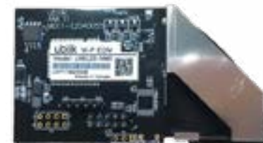
Figure 4: Ubiik's FAN communication device.
